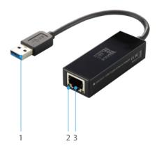
1. USB 3.0 Connector 2. LED Indicators 3. RJ-45 Ethernet Port
